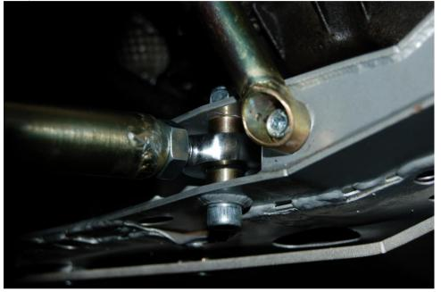
Fit the subframe to body braces next. There are four braces, all of which are different. Three of them fit to the standard holes in the body and one will need a rivnut fitting. Fit the three others first using M10 bolts at the subframe and M8 bolts on the body.
