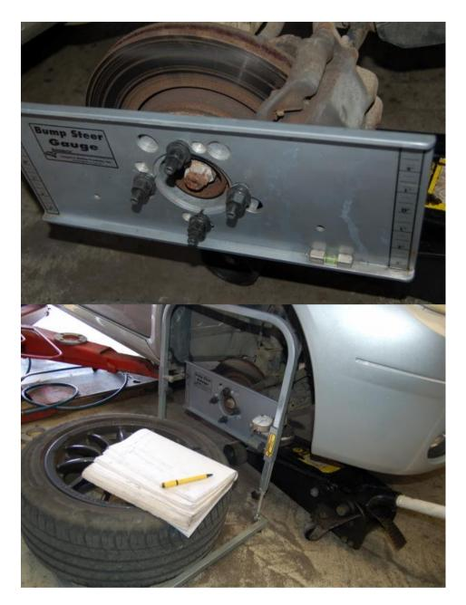
If you have a very different track width from standard you may need to reduce the upper spacer thickness instead of increase it – if this is the case, swap the small lower spacer with the upper one and use shims as necessary above the small spacer.
