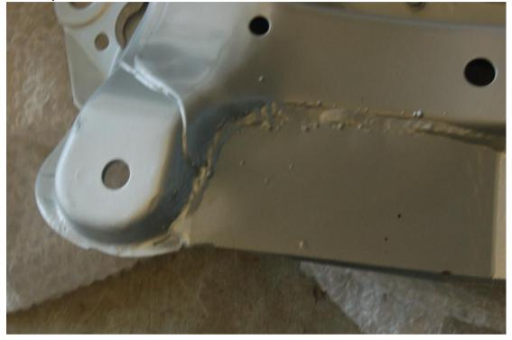
Once you can slot the stiffener in, align it using the holes in the stiffener and the holes in the subframe.
