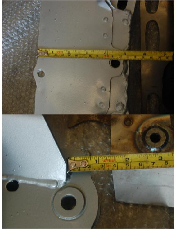
Once you are happy with the alignment, weld the stiffener in place around all edges and in the oval cut-outs on the top.
