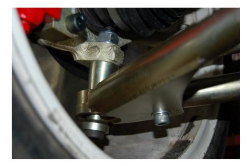
Fit the bump steer kit to the track rod: Remove the front springs (if already fitted) and track rod ends.
