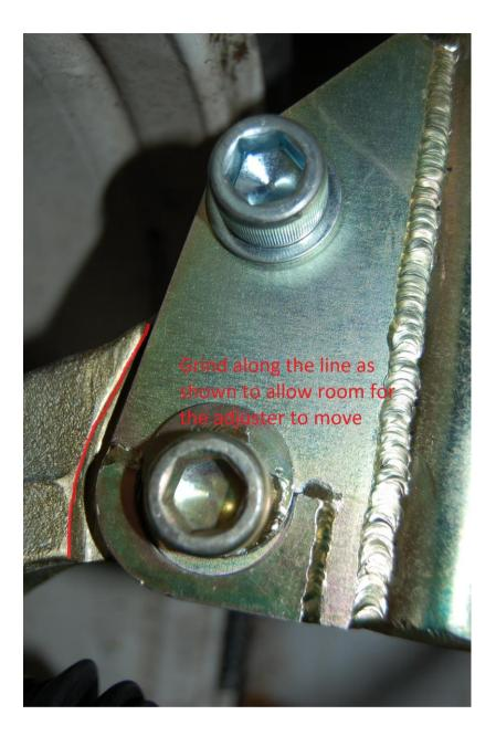
Fit the spacers and bolt (as shown below) to the outer joint. Torque M14 bolt to 165Nm.
