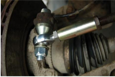
Depending on how wide your front track width is, you will probably find that the track rod is too long to get back to parallel toe. If this is the case cut a few threads off the end of the track rod with a thin disc in an angle grinder.
