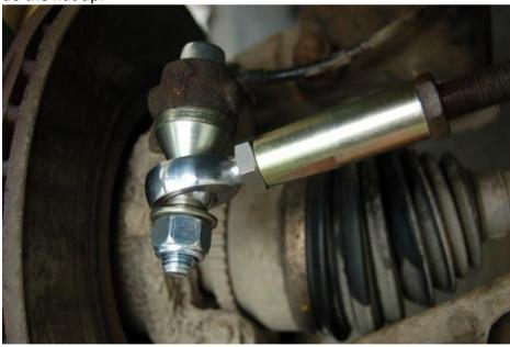
Set front toe to desired setting or close to parallel for the bump steer set up procedure.
