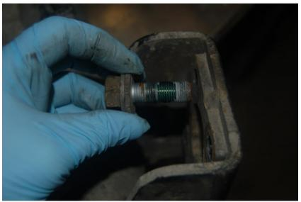
Refit stub axle bolts and torque to 105Nm.
