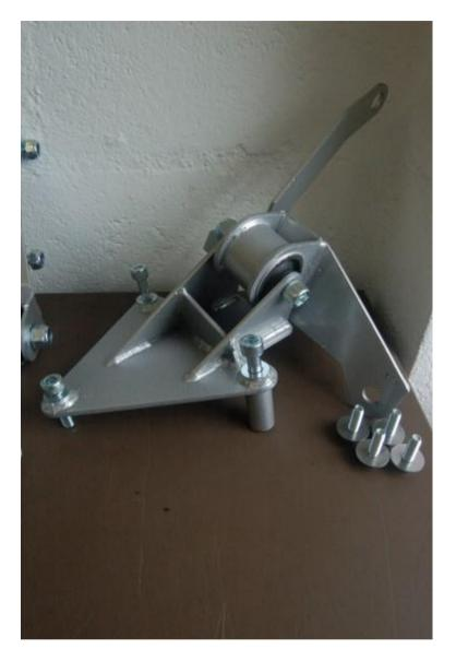
Fit up the body side of the upper gearbox mount, slotting in the polyurethane thrust washers on either side of the bush and use the M12 bolt, washer and nyloc. Fit the M8 bolts into the body with penny washers and torque to: M8 25Nm, M12 to 116Nm.
