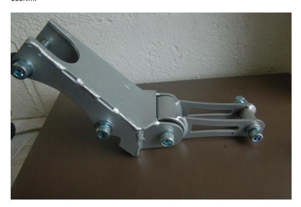
Hold the engine/gearbox in place with suitable lifting gear or jack under the gearbox. Remove the upper gearbox mount from the gearbox and the body. Bolt on the new gearbox side of the mount using the three M10 bolts and washers – torque to 60Nm.
