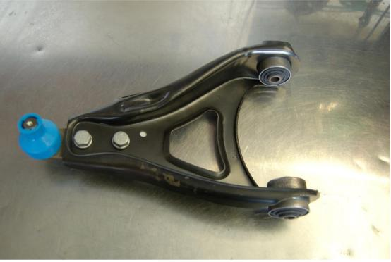
Press out the bushes using a suitable tool.
