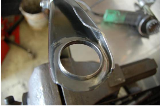
The following paragraph is updated due to variations in the wishbone bush spacing: Press in the front housing from the inside until it bottoms out on the shoulders and tack in place. Now either:
