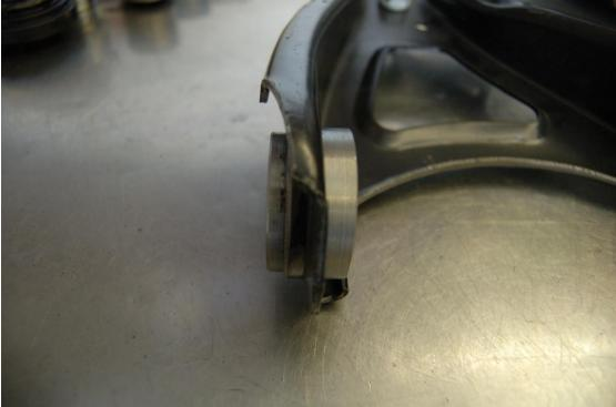
Weld all around the housings (Please note: the housings are made so that they will shrink to the correct size after welding to give the bearings a light press fit)
