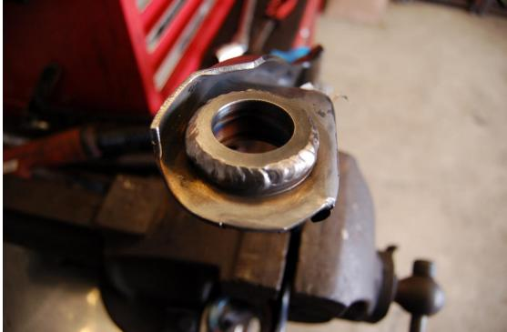
Remove the powder coating from around the top of wishbone and rest the plate on the top using an 18mm socket on the ball joint bolt to locate the access holes properly.
