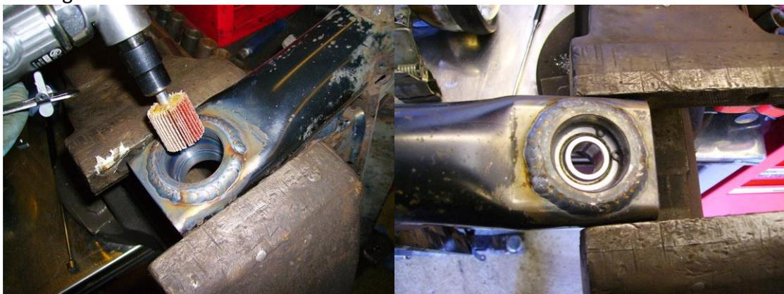
Push the axle back into place and bolt back up using the original bolts (we do recommend the use of new nuts), (You may have to slacken off the bolts on the axle – body mounts to get the bearing spacers to fit)
