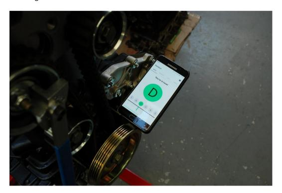
Using a new bolt, liberally coated in Loctite 243, tighten crank pulley bolt to 40Nm + 110 degrees.
