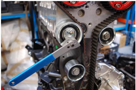
To measure tension very accurately we use a guitar tuning app on a smartphone and tune by 'plucking' the longest front section of belt to an 'A' 110hz for hydraulic lifter engines and a 'D' 146hz for solid lifter conversions with stiffer valve springs and longer durations cams. This may seem tight but once bedded in the belt relaxes very quickly. Torque tensioner retaining nut to 28Nm.
