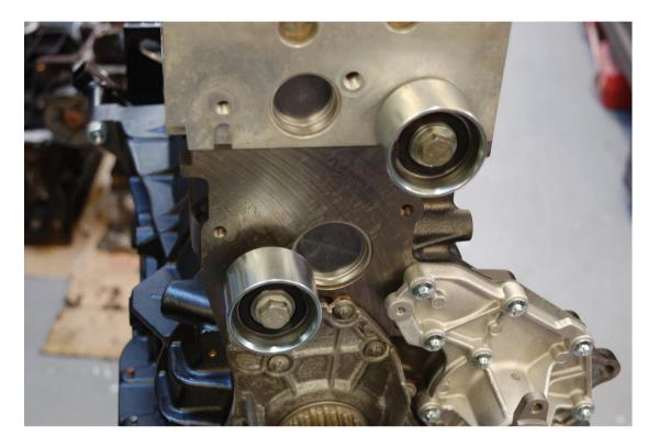
Make sure the camshaft locking tool is in place.
