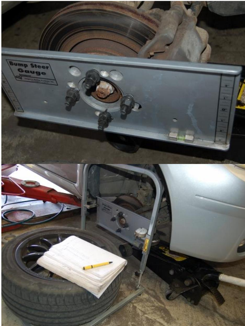
If you have a very different track width from standard you may need to reduce the upper spacer thickness instead of increase it – if this is the case, swap the small lower spacer with the upper one and use shims as necessary above the small spacer.
