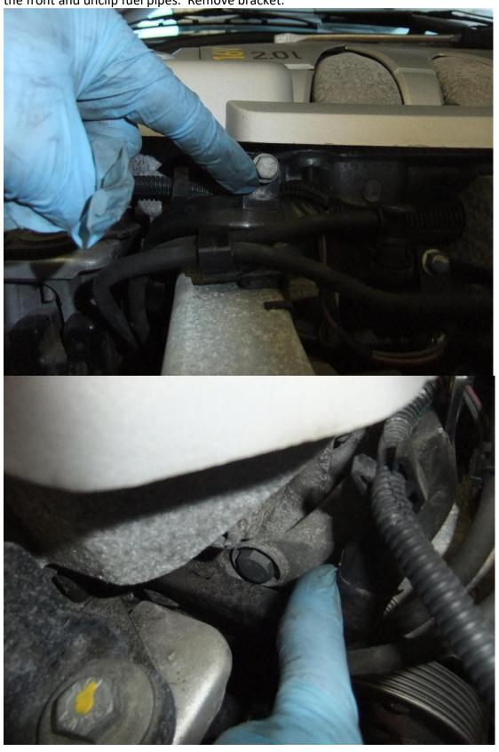
Refit the 16mm and 13mm bolts back into the inlet manifold.
