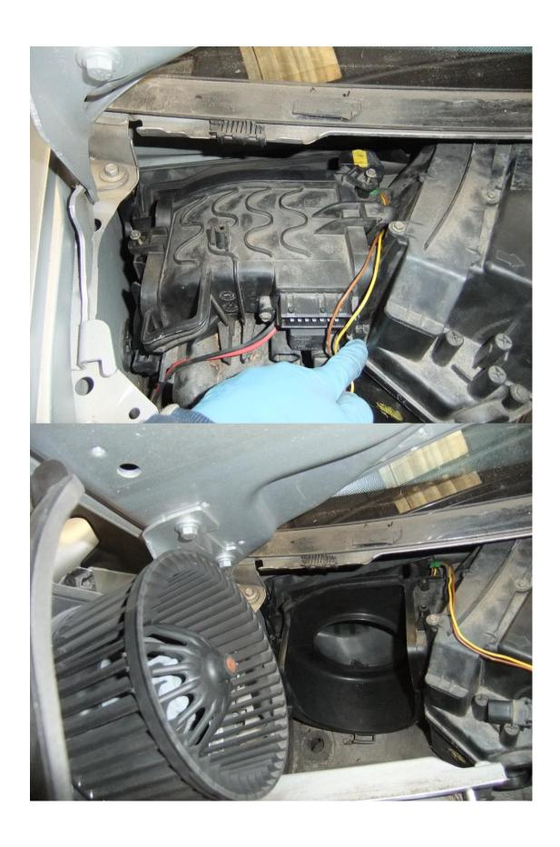
Remove the two 10mm bolts that hold the centre air duct in place and pull the duct towards the NS of the car.
