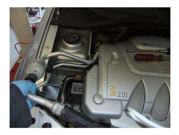
Disconnect the alternator wiring and remove the alternator top bolt. Slacken the bottom alternator bolt and swing the alternator forward. Remove the alternator bottom bolt and pull the alternator out.
