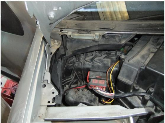
Remove the clips holding the sound deadening to the bulkhead and pull it forwards. Remove the top two bolts and the NS bottom bolt from the heater cover panel, slacken the two bottom bolts and pull out the panel.
