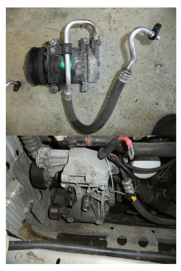
Remove the alternator support bracket.
