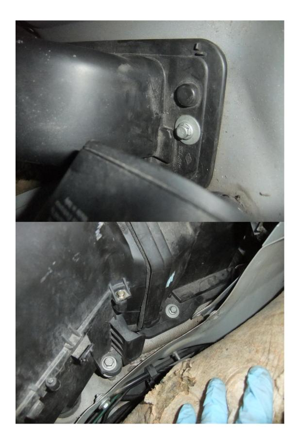
Remove one bolt in the scuttle and the two bolts behind the dash in the driver's foot well that hold the main casing in place. (The bolts aren't quite shown on this picture but they are low down at either side of the bulkhead opening)
