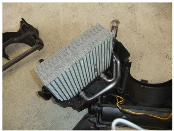
Cut out a piece of plastic to fill in the hole that is left in the unit and bond in before putting the unit back in the car. (There is positive pressure inside the unit when the fan is on so bond the plastic into the outside edge of the casing)
