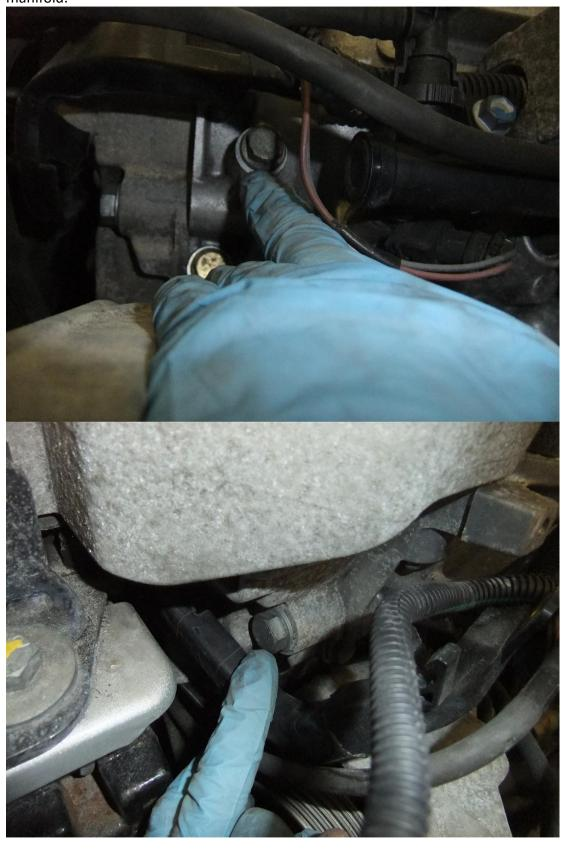
Remove the fuel pipe clip from the top alternator bracket by pulling out the centre dowel as shown.
