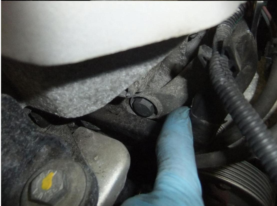
Refit the 16mm and 13mm bolts back into the inlet manifold.
