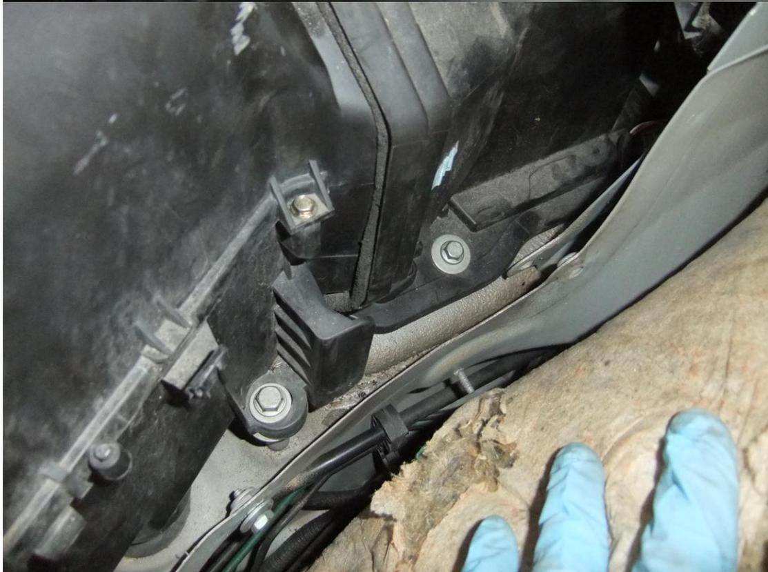
Remove one bolt in the scuttle and the two bolts behind the dash in the driver's foot well that hold the main casing in place. (The bolts aren't quite shown on this picture but they are low down at either side of the bulkhead opening)
