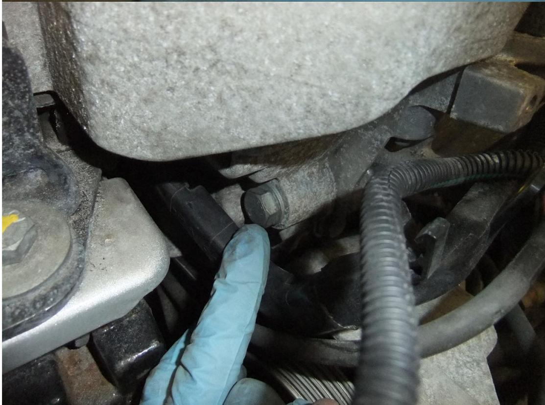
Remove the fuel pipe clip from the top alternator bracket by pulling out the centre dowel as shown.
