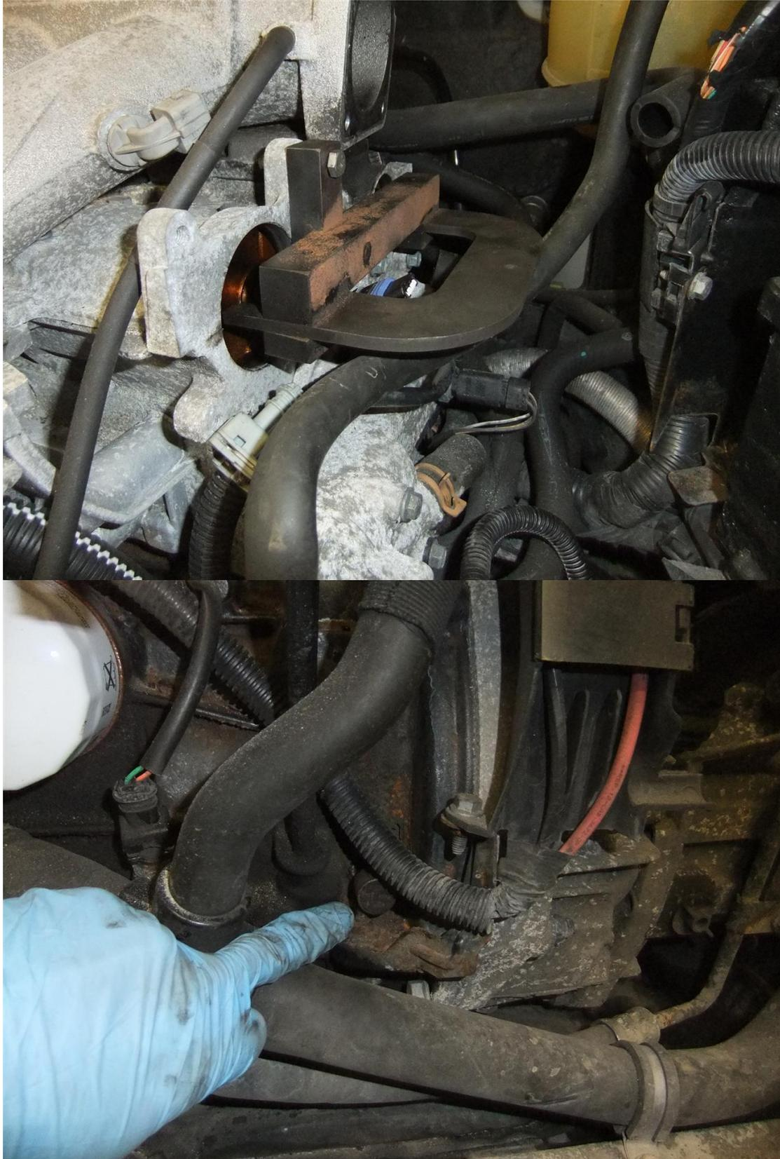
Lock the flywheel using a large screwdriver or similar, slacken and remove the crank pulley bolt and pulley.
