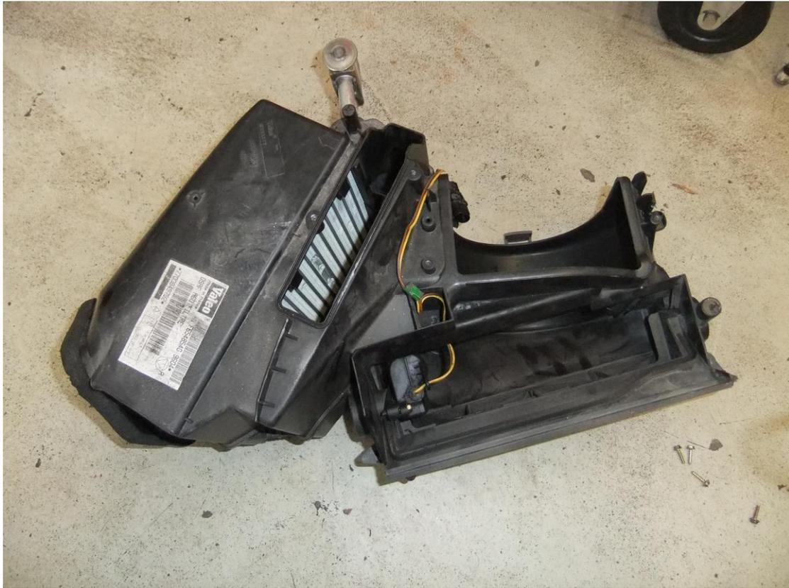
Remove the recirculation flap motor and all screws holding the two halves together.
