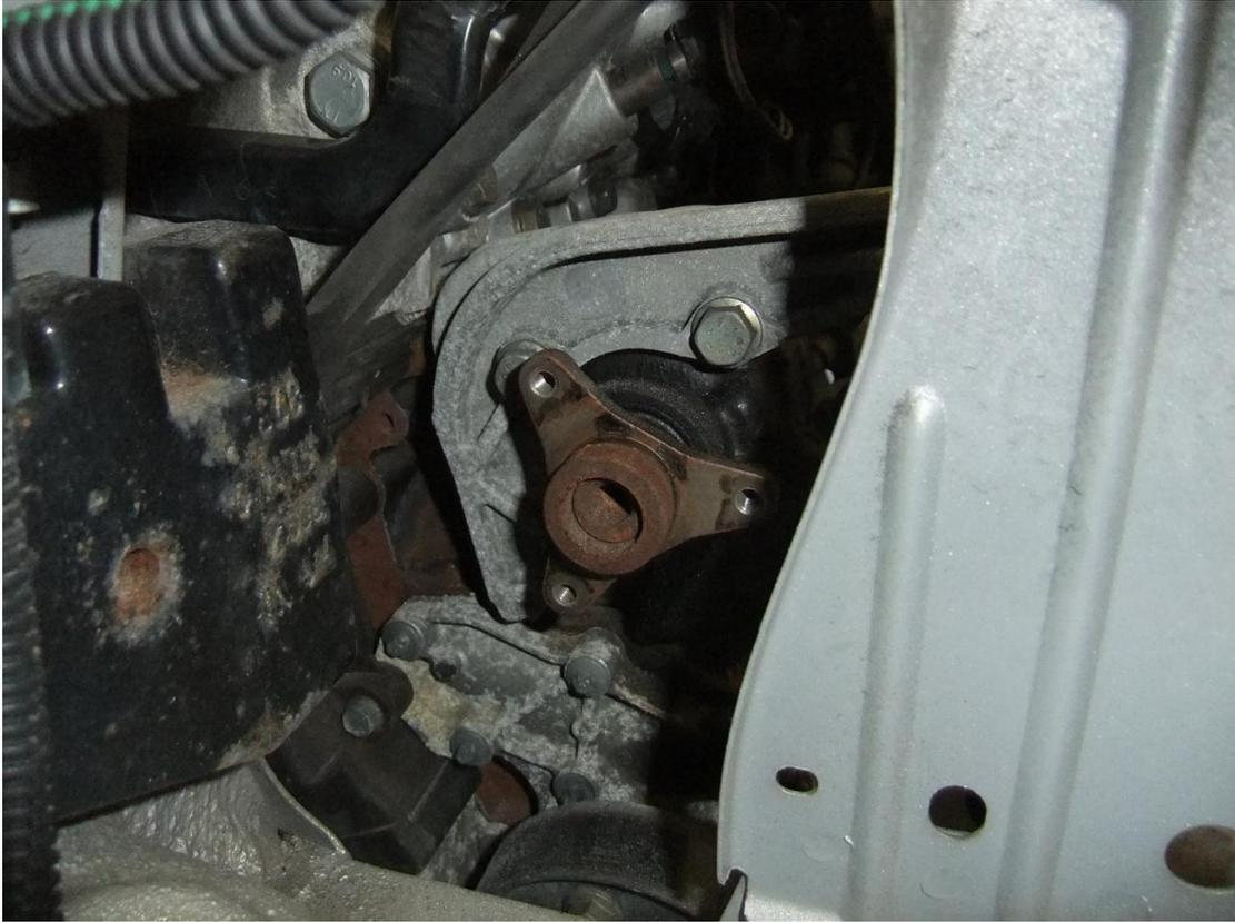
Remove the water pump pulley, clean spindle and fit new pulley using loctite on the M8x16mm bolts.
