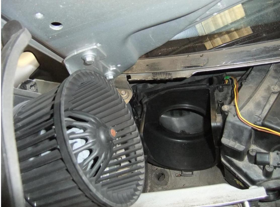
Remove the two 10mm bolts that hold the centre air duct in place and pull the duct towards the NS of the car.
