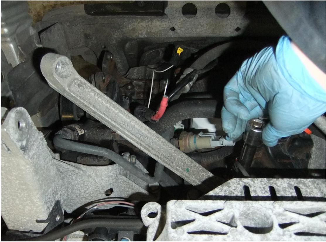
Remove the engine cover, MAP and VVT solenoid wiring plugs, the 10mm bolt holding wiring loom in place and push wiring aside to gain access to 16mm bolt. Remove 16mm bolt from the side of the top alternator bracket, the 13mm bolt from the front and unclip fuel pipes. Remove bracket.
