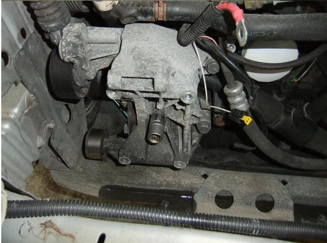
Remove the alternator support bracket.
