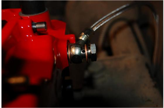
Fully remove the original brake flexi hose, retaining the original spring under the brake pipe fitting. Fit the new flexi hose quickly to minimise fluid loss. Goodridge recommend a torque of 19 to 32Nm.
