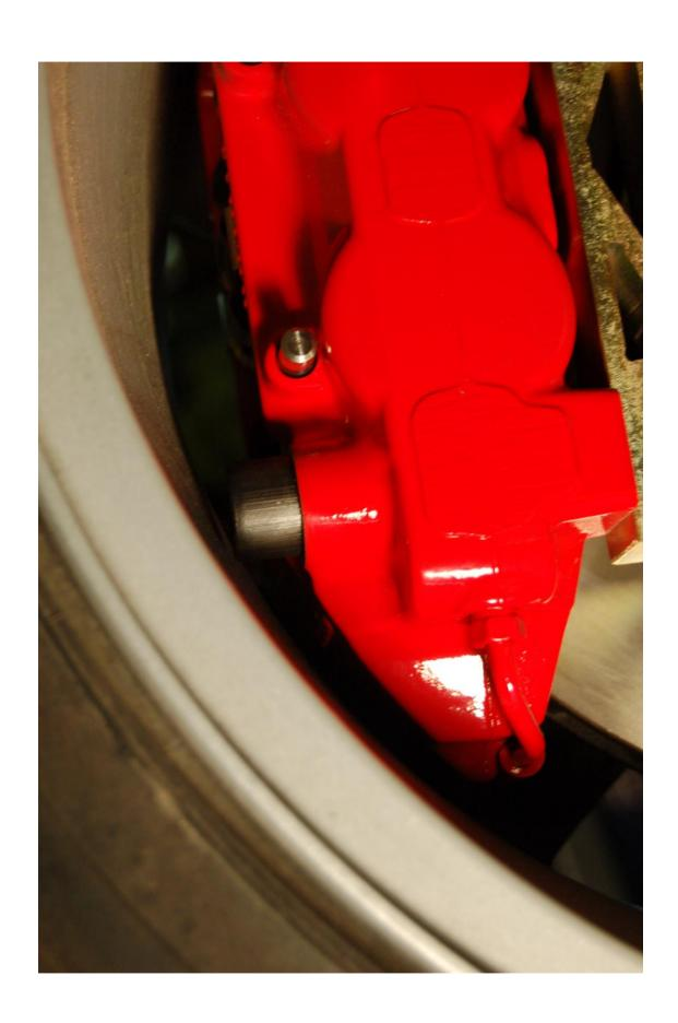
Fit the brake pads and springs using the pins as shown. Use some grease on the pins
