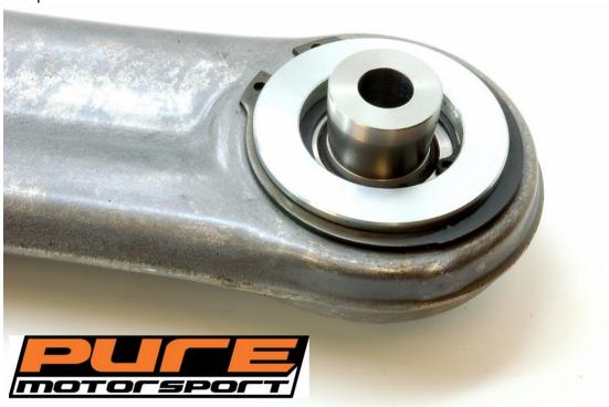
Press the front housing into the wishbone from the front so that the flange sits against the machined face of the wishbone.
