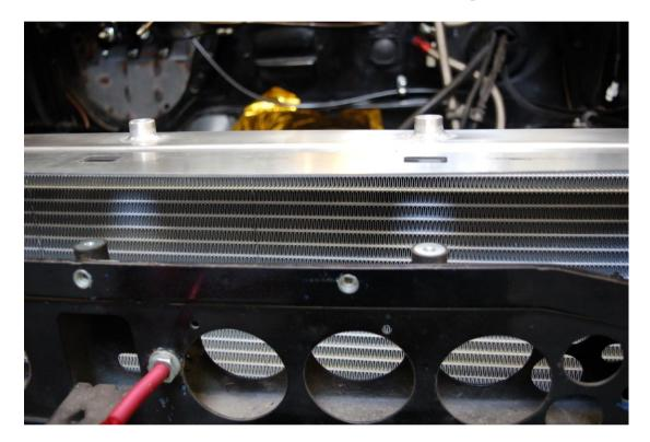
Fix the upper straps using Loctite on the M6x12mm bolts and penny washers and adjust so that the radiator is clear of the bodywork.
