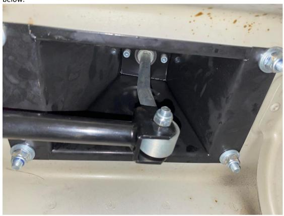
Now go back to the engine bay and first job is to fit the captive stud. There is a hole in the chassis rail below the ABS modulator. Leaving the nut on the stud, and making sure the castellated washer is fitted underneath the nut, push the stud into the hole, hit the end of the stud with a hammer until it is flush with the end of the thread. Follow this link for more information: <a href="https://www.blindbolt.co.uk/heavy-duty-">https://www.blindbolt.co.uk/heavy-duty-</a>
