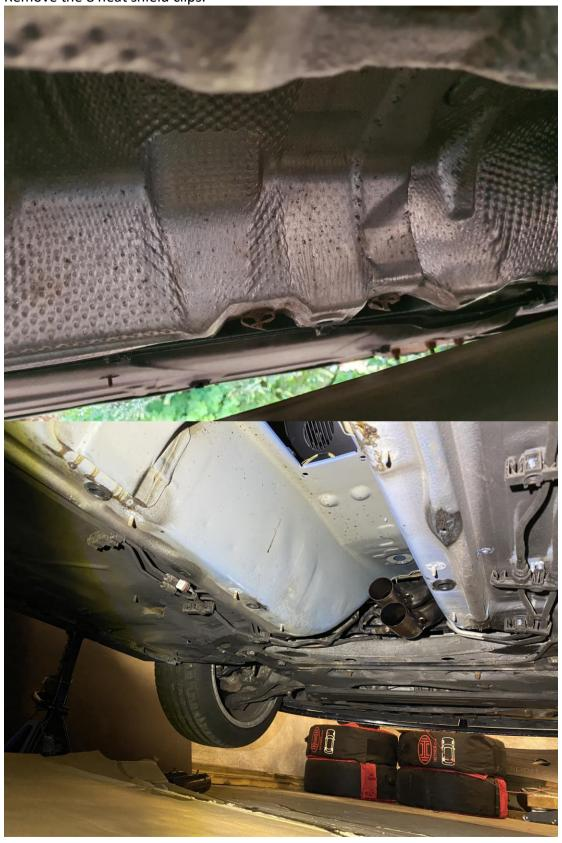
Pull heat shield towards the back of the car and remove.
