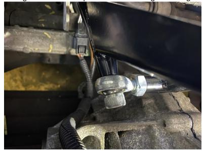
Then fit all of the linkage rods at the front as shown below. When fitting the ball joints remove the clips before pushing on and fit them after you have finished setting the linkage up – do not lose the clips as they aren't available separately and you will need to purchase a new ball joint!
