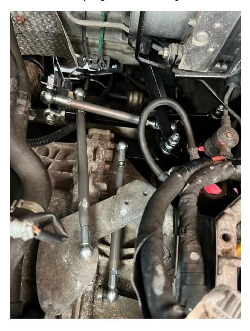
Finally remove the bolt at the bulkhead side, underneath the ABS modulator and fit the strap from the bellcrank bolt to here, reuse the original bolt.
