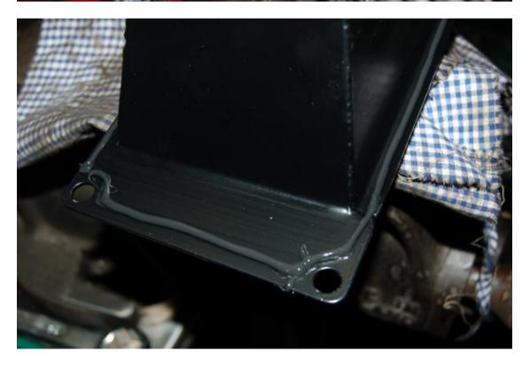
You will need to get a glamourous assistant to help you to fit the tower from underneath the car. Hold the tower in place and <u>push towards the rear of the car</u> as far as it will go, bolt into place with the bolts and washers going in from above and washers and nuts below.
