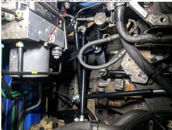
Using Loctite on the M10 bolt, fit the lower rod to the M10 rod end on the 'A' arm and tighten with the help of someone holding onto the gearstick inside the car.
