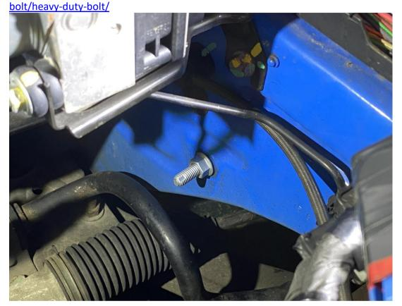
Remove the nut, making sure not to push the stud into the chassis or you will lose it! The castellated washer should hold it in place.
