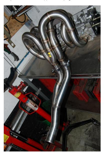
Ensure that all engine bay components are suitably protected with heatshield material. Do not wrap the exhaust in anything.
