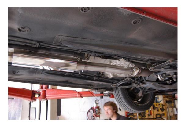
Fit the centre section to the decat or cat, push the rod into the rubber mount and partially tighten clamp.
