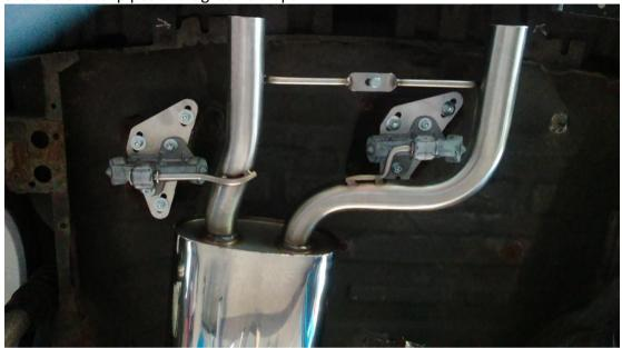
Use a pair of our carbon trims to make a very neat finish to your rear bumper. Tighten up the rear mountings when happy with the fitment. Adjust as necessary. Swap the lambda sensor(s) over and plug them back in.
