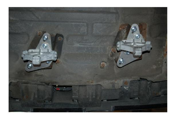
Now fit the rear silencer, sliding the rods into the rubber mounts and fitting the penny washers and bolts.
