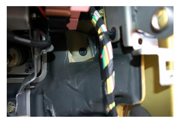
Push a sharp point through the grommet to open a little hole.
