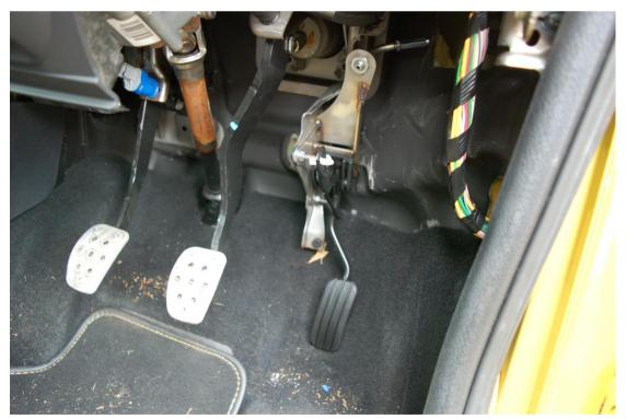
From the footwell push the outer sheathing of the cable through the grommet and extract it from the engine bay side and pull through into engine bay until you have about the right length left in the footwell. Push the sheathing into the 90 degree fitting on the pedal bracket and into the throttle bodies. Trim the outer sheathing
