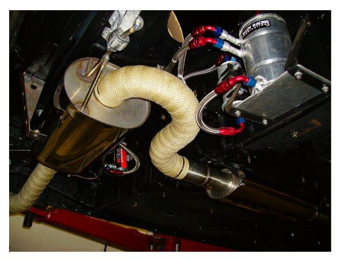
Ensure that the connection pipes are correctly mounted and do not pull tight with engine movement. Spigot-ended fuel rails are only 8mm diameter under the hose - insufficient to restrain an engine without breaking! Ideally use a fuel swirl pot fuel system arrangement to ensure there is always
