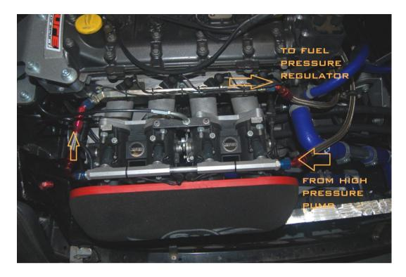
We recommend using a fuel pressure regulator fitted as close to the engine as possible but isolated from engine vibration and heat.
