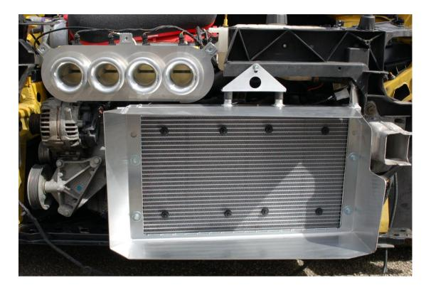
Fit our radiator pack into the original rubber mounts, adjust and bolt up the top radiator bracket. Using all the standard hoses and clips, refit the coolant hoses. Reroute the top expansion tank hose under the filter backplate and clip back to ensure it doesn't chafe on anything.
