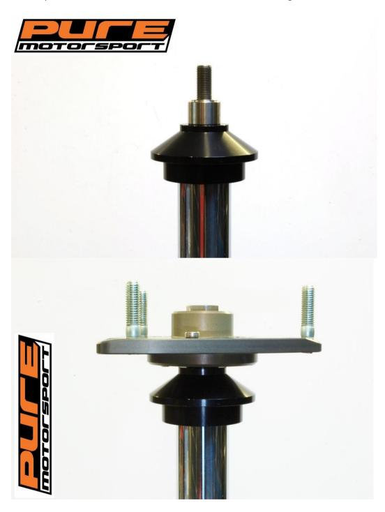
If you want to use maximum camber settings and place the top mount further back to get maximum caster setting you may need to remove the lip on a portion of the strut top as shown below. It is only the lip that needs to be removed.
