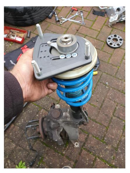
If you have coilovers with parallel springs then fit our stainless steel lower spacer, then top mount and then use Loctite on the sleeve nut and tighten.
