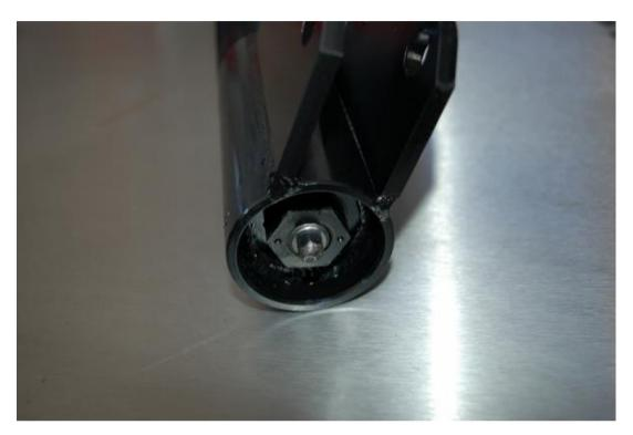
Rear dampers are adjusted by using the knob on the base of the unit.
