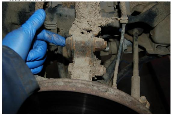
Do not touch the grub screw in the top of the front struts – this covers the valve used for gassing the units.
