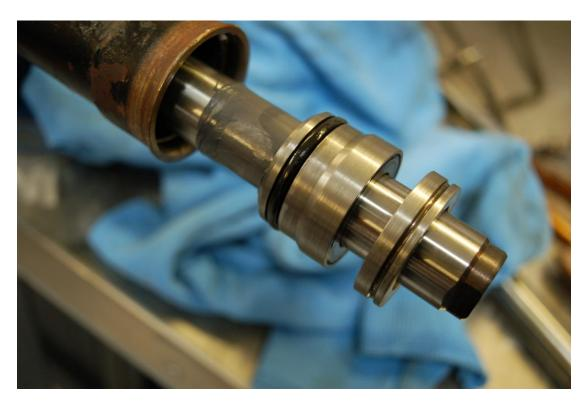
Push the end bush and plug back onto the casing until the clip recess is lined up with the cut-out in the casing.
