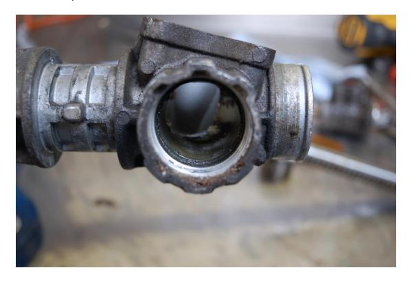
Clean the new rack and pinion. Cover the rack and inside the casing with high quality grease suitable for highly loaded components.
