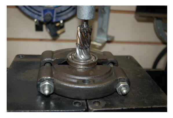
Put the seal on the new pinion, press on the bearing and put the circlip in the groove.
