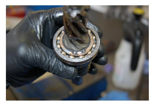
Press the bearing off the pinion.
