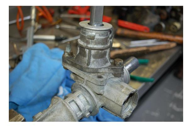
Grease the rack at the base of the preloading bush.
