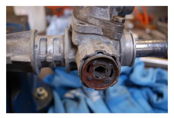
Plug the hydraulic ports to stop water and dirt ingress by using our plug kit available to purchase separately.
