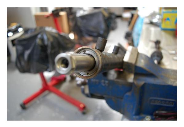
Rotate the rack end plug using an appropriate tool (long nose pliers work OK) until you can see the end of the retaining clip.
