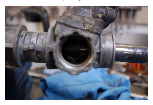
Push the pre-loading bush back in with spring and washer.
