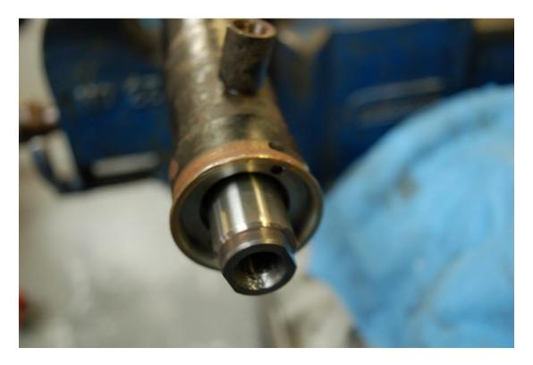
Turn the end plug until you can see one of the holes for retaining the end of the clip. Push the clip in the hole and turn the end plug until the clip is fully seated in the groove.
