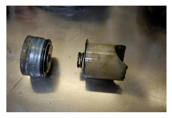
The casing should now be bare. Clean inside and outside the casing, paint the steel section if required.
