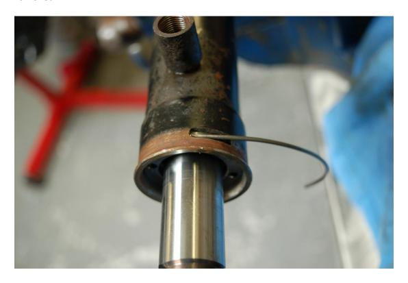
Hold end of the rack in a vice, cover the hydraulic ports so that you don't get covered in fluid and pull the casing away to remove the rack.
