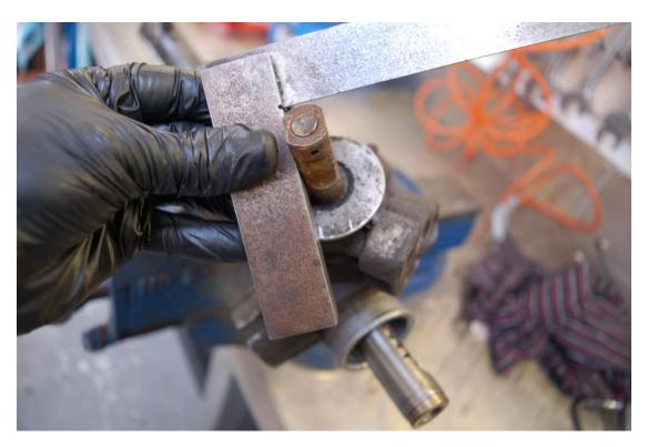
Remove the two bolts from the pinion housing.
