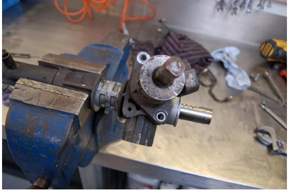
Remove the pinion and housing.
