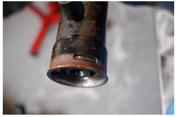
Tap the top of the pinion until the bearing, seal and pinion come out of the housing.
