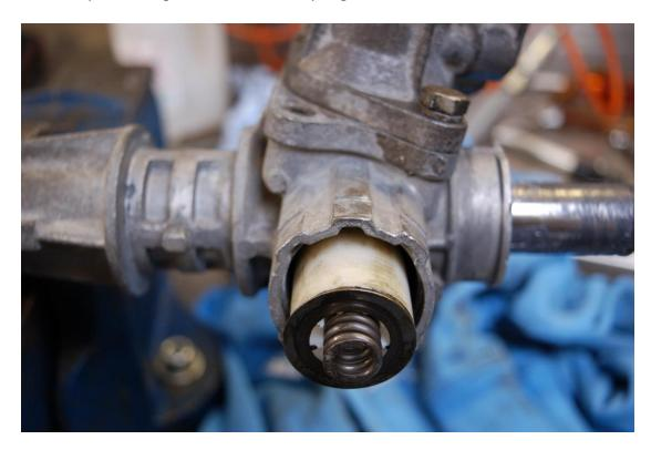
Fit the screw on cap, tightening until there is slight resistance felt when rotating the pinion. There should be very little or no rotational play in the steering rack. Using an adjustable spanner work the rack from lock to lock making sure the movement is smooth with no excessive notchiness. Recheck the pre-loading and adjust if necessary.
