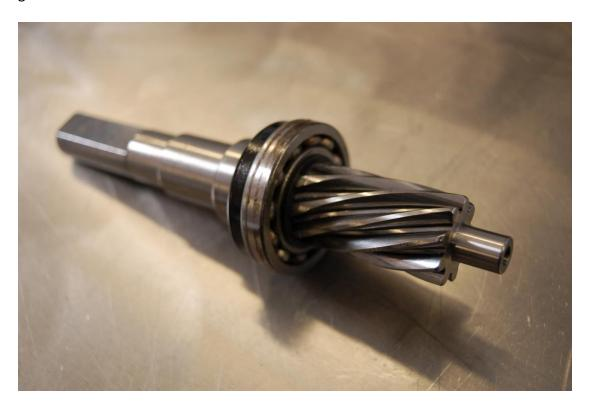
Clean the pinion housing, grease the inside and press the bearing and pinion back into the housing.
