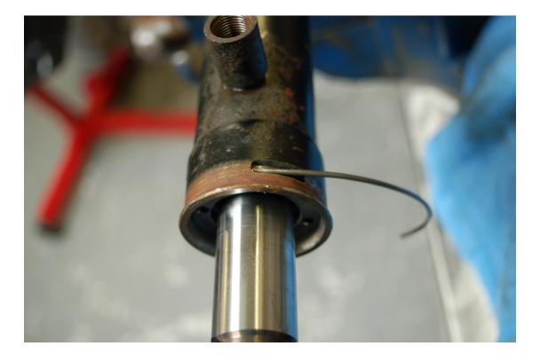
Turn the plug in the opposite direction until both ends of the clip are no longer visible,
