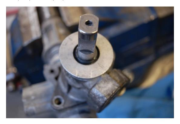
Taking care to keep the rack centralised, push the pinion back into the rack casing ensuring the pinion remains lined up with your marks. Bolt the pinion housing back on.
