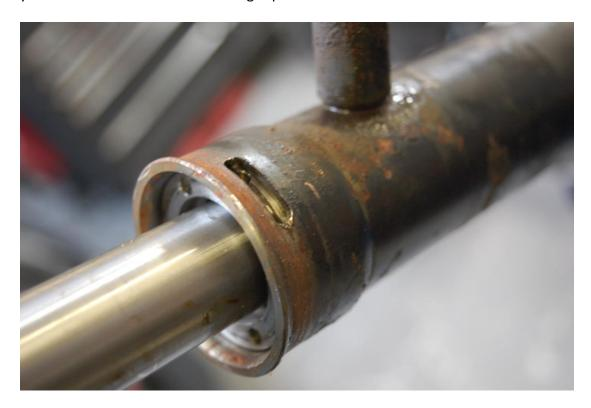
Pick the end of the clip out of the casing and rotate the end plug until the clip can be removed.
