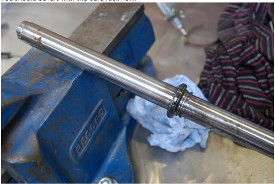
Prise out the retaining ring indentations and unscrew the rack and pinion pre-loading bush.
