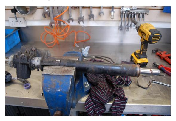
Using Vernier callipers centralise the rack until you get an equal measurement of rack protrusion on each side of the rack from the end to the inside of the casing where the lock stops bottom out.
