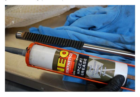
Slide the rack back into the casing spreading the grease around all the bushes.
