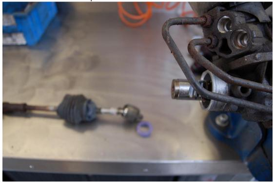
Remove the hydraulic pipes.
