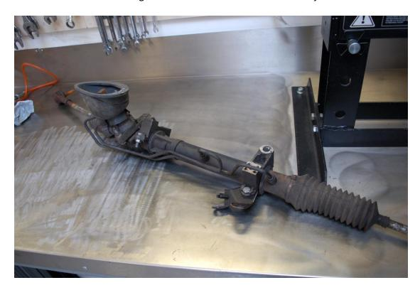
With the steering rack held in a vice, snip the inner track rod joint gaiter clips and pull back the gaiters. Using a suitable spanner or the correct Renault removal tool unscrew the track rods and put to one side.
