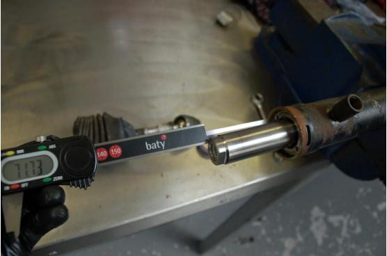
With the rack centralised, mark the position of the pinion on the pinion casing with a scribe or similar. Mark on the side of the recess in the pinion for the steering rack clamp bolt so you don't get the pinion the wrong way around!
