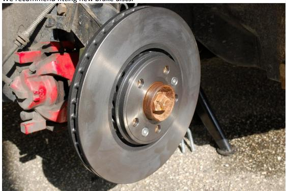
Fit the brake callipers using loctite on the M14x1.5 bolts. Torque to 170Nm. Fit the brake pads and springs using the pins as shown. Use some grease on the pins to stop them sticking and tap them into place.
