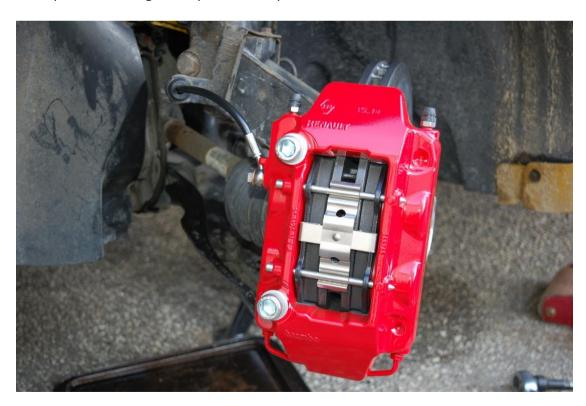
Fit the calliper end of the flexi brake hose using the copper washers provided on either side of the brake banjo. Goodridge recommend a torque of minimum 19Nm.
