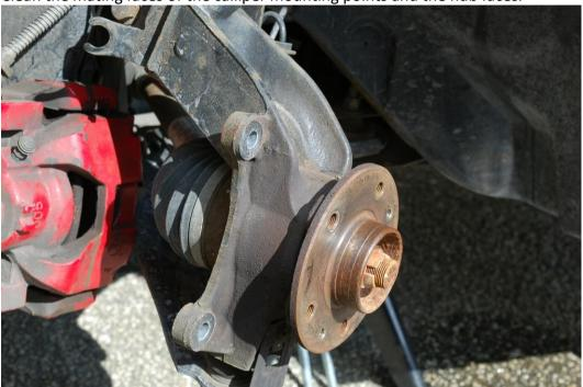
Fit the new brake calliper brackets using the M12x1.5 bolts and K Nuts. Torque to 100Nm.
