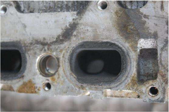
There are some cylinder heads with very thin castings between the exhaust port and water jacket. Please measure the depth of the water jacket (as shown) on a head that hasn't been skimmed. The maximum acceptable depth is 13.5mm.
