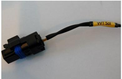
VVT solenoid plug – is male, two pin plug – to plug directly into the standard Renault VVT solenoid.
