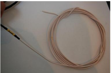
Fuel pump +ve feed from fuel pump relay - includes a long single wire for connection directly to the positive terminal of the fuel pump.
