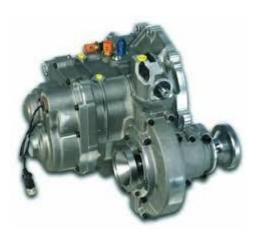
Full throttle gearshift capability. Includes wiring tails to connect to existing gearshift switch/load cell and wiring tails to connect to existing gearshift barrel position sensor.
