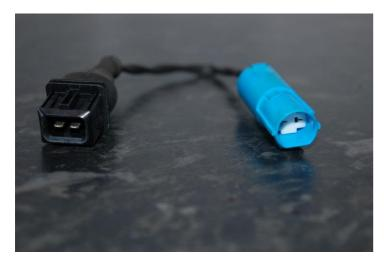
Crank sensor sub loom, male mini timer plug (to suit loom connector) to blue Renault TDC sensor plug. You must ensure you use the new style crank (TDC) sensor from Renault with the blue plug on the top.
