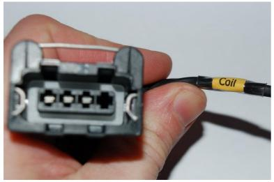
Ignition coil plug has a four pin female mini timer plug – to plug directly into the standard Renault coil.
