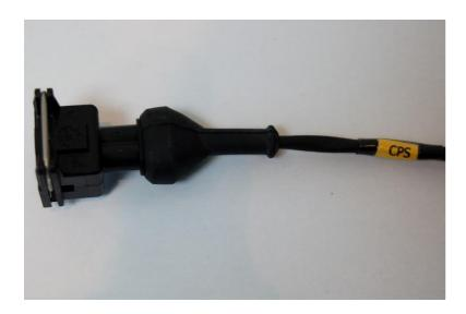
Crank position sensor has female mini timer plug – to plug directly into our crank (TDC) sensor sub-loom
