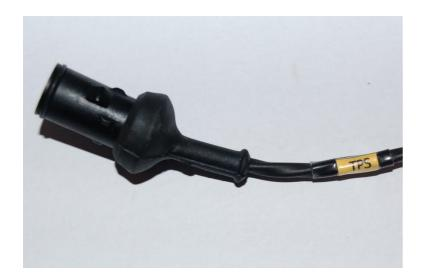
Throttle position sensor is a three pin male plug – to plug directly into the Colvern type TPS supplied in our sensor kit.
