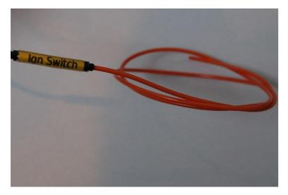
Ignition switch +12v for controlling ECU and fuel pump relays – plain cable end.
