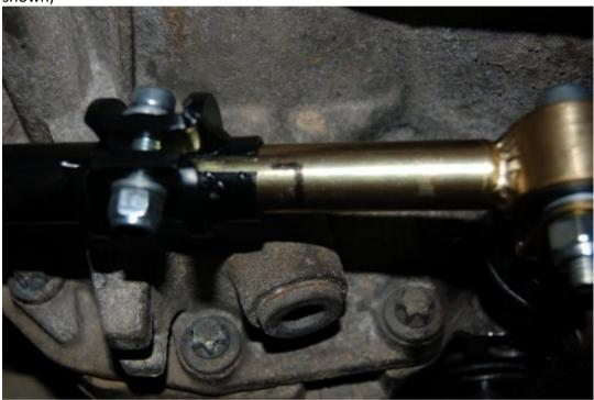
This is your starting position for clamping up the linkage rod.
