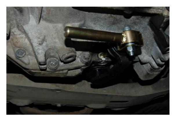
Join the link rod to the front pivot, don't clamp up yet.
