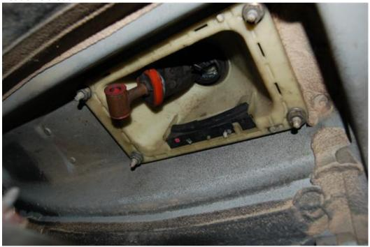
Remove the four 13mm nuts holding the tower in place and remove the tower,
