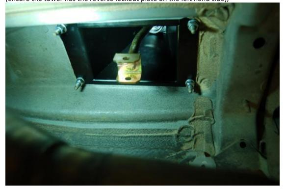
Put the exhaust heat-shield back into place but don't fasten. Place the new link rod through the hole in the heat-shield with the bearings to the rear. Fit the new link rod making sure the stick is in the correct orientation with the stick kicking backwards. Fix using the M10x45mm bolt and shallow nyloc nut, placing the 10mm spacer washers to fill the gap between the clevis and the bearings.
