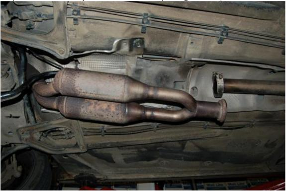
Remove the fasteners holding the front exhaust heat-shield in place and drop the heat-shield to access the gear linkage tower,
