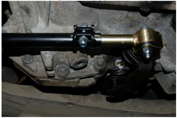
Refit the exhaust heat-shield and fold back some areas around the linkage rod hole until the rod has enough clearance.
