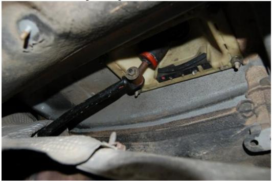
Remove the 13mm nut holding the linkage rod in place, remove the rod and pull the heat-shield out.
