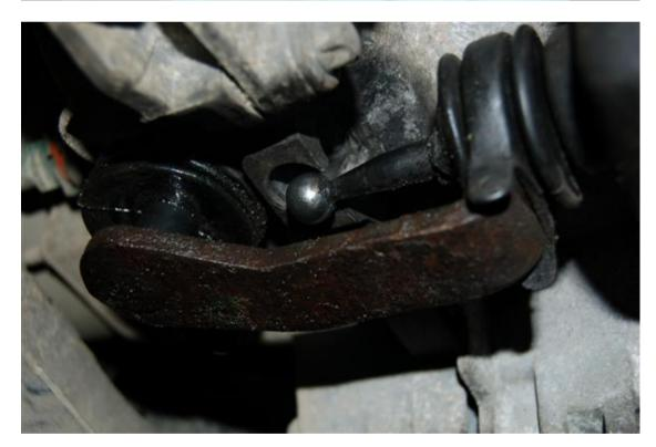
Pull the pivot out of the rubber gaiter,
