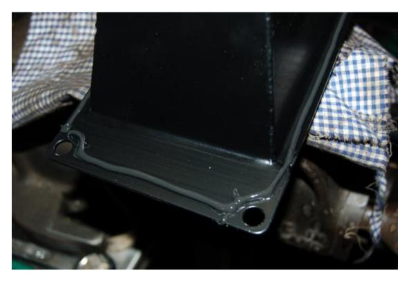
Put the new tower and place and fix using the four 8mm nyloc nuts and washers (ensure the tower has the reverse lockout plate on the left hand side),
