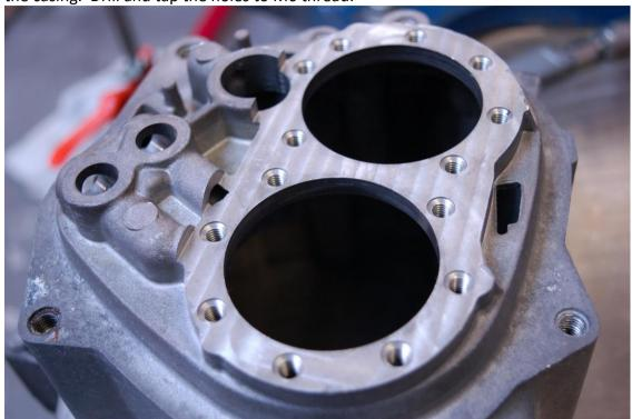
After cleaning the casing thoroughly; Add Loctite to the mounting face, bearing outer races and M6 bolt threads and fit the plate torqueing M6 bolts to 6-8Nm.
