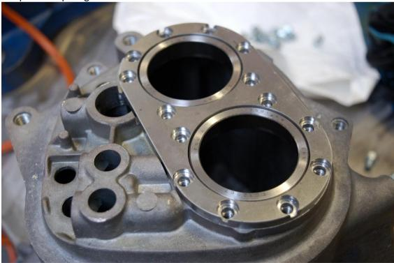
To clear the new plate you will need to grind reverse gear shaft down flush with existing cut out making sure it extends at least 31mm to the start of the radius as shown below. Ensure the reverse gear shaft clears the plate when reassembling the gearbox.
