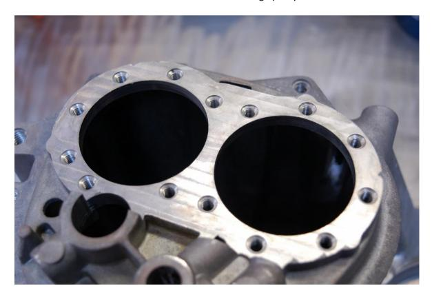
Offer up the reinforcement plate ensuring it is the correct way around taking into account the different hole spacing around the reverse gear shaft hole and fit the bearing outer races to hold the plate in place. Transfer punch the hole centres onto the casing. Drill and tap the holes to M6 thread.
