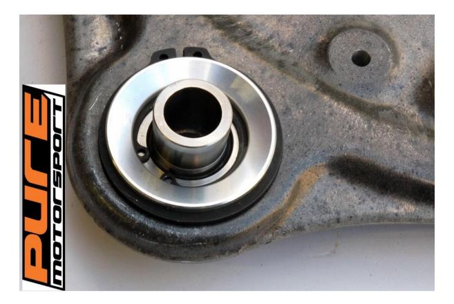
Fit the stainless spacers and refit the wishbones to the car.
