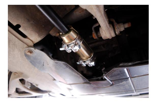
If you find that the mass damper touches any parts of the subframe or engine mount with it mounted further forward it can also be mounted as shown below.
