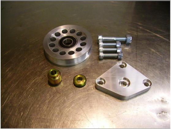
Continue with pulley kit fitting or if our pulley kit is already fitted then refit and tension auxiliary belt.
