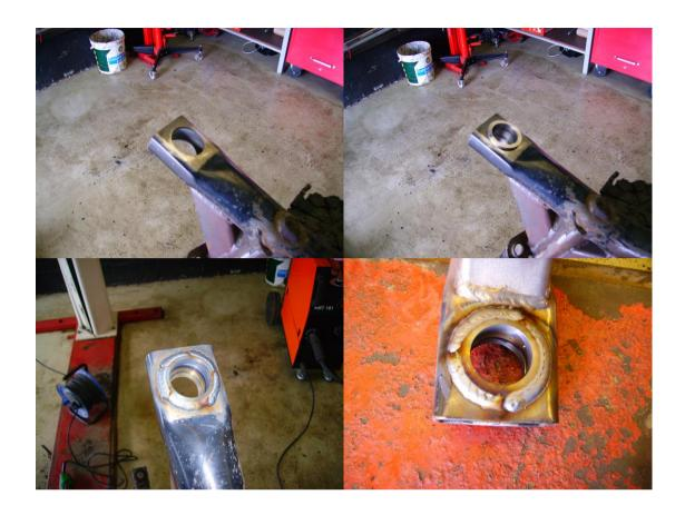
Paint the axle if you wish and then clean the inside of the housing using a flap wheel to remove any weld spatter or paint. This is just to clean it not to make it bigger so go easy!!
