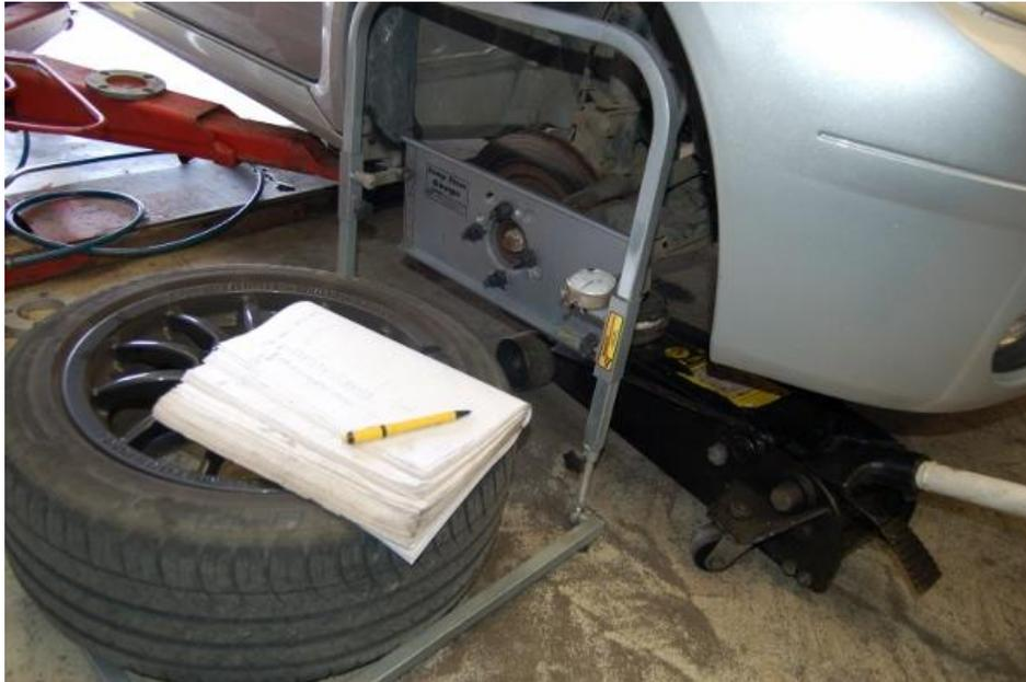
Once you are happy with the bump steer set up, refit all the components, torque rod end bolt to 116Nm.
