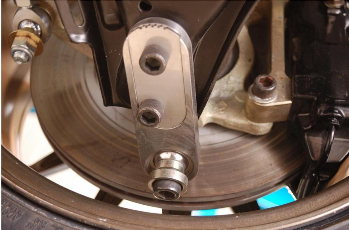
If you are using a front anti roll bar you will need to cut off the front corner of ARB clamp to clear the new spherical bearing housing.
