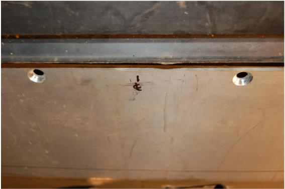
Offer up the sump-guard so that the fold is in a position to offer the best fit.
