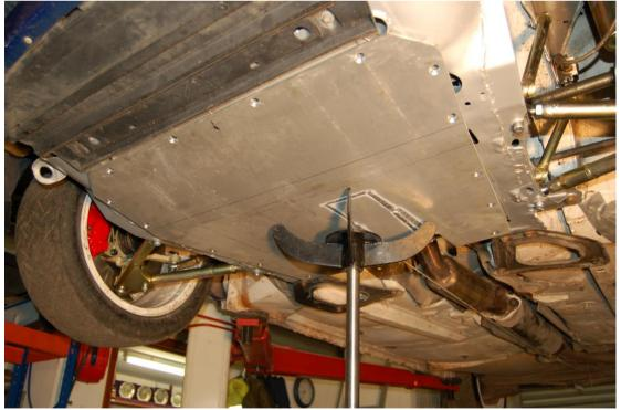
• If you are fitting to a car with a Renaultsport Clio Cup race car subframe you will have to remove some material around the engine mounts.
