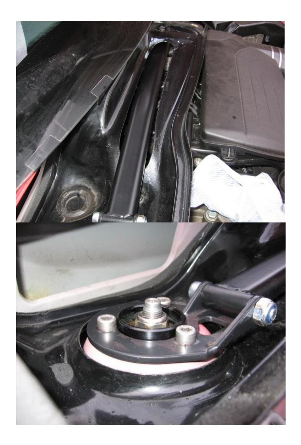
Using gaffer tape, cover up the gaps between the heater intake panel and the brace to stop any water running through as shown.
