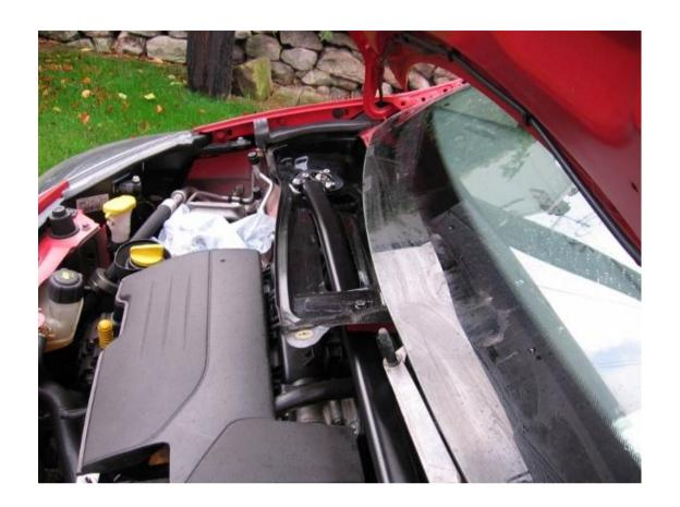
Loosely assemble the strut brace with the mounting lugs forwards, with the bent side of the bar on the right hand side of the car and place onto strut tops. Centralise the centre holes at each end and mark the three mounting holes on the strut top with a scribe or pen. Remove brace, centre punch and drill the holes to 8.5mm. Check fitment of the top mounts and brace, adjust if necessary. Brush some paint around the holes to cover the bare metal, leave to dry.
