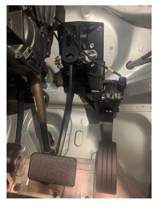
Plumb in the brake pressure side using a front/rear split and a rear bias valve can be used in conjunction with this bias box.
