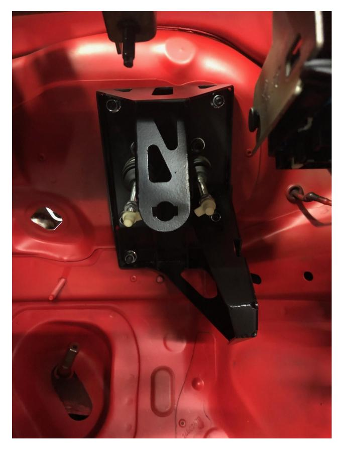
Mark and drill two holes in diagonally opposite corners and ensure the pedal box is level and square. Drill the remaining holes through the bulkhead but do not bolt up at this point. Mark the centre holes of the two master cylinders and use a very small
